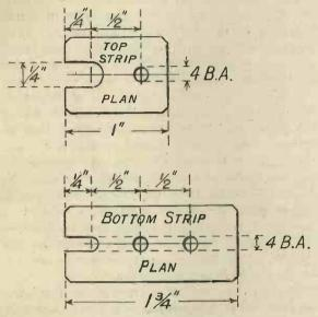
Fig. 2. Details of brass strips.
