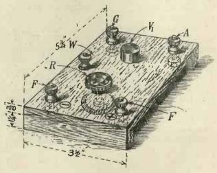
Fig. 11. Illustrating a suitable valve panel.
