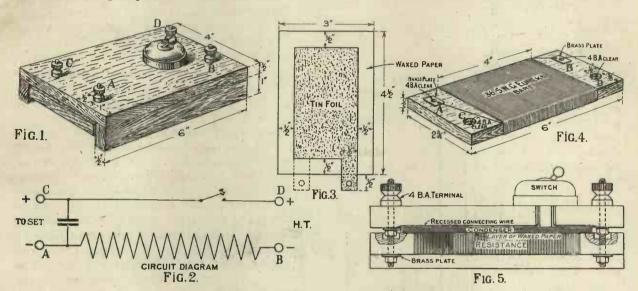
Figs. 1-5. Showing constructional details of the safety unit.
