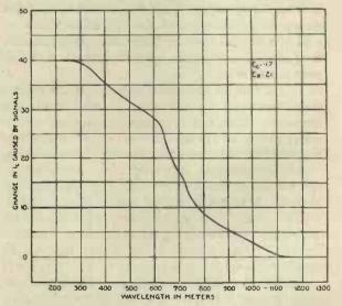
Fig. 4. Curve showing the change in collector current for impressed signals at various wavelengths.
