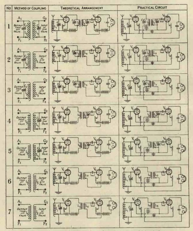
Fig. 1. Diagrams illustrating the various types of intervalve couplings and their mode of use.
