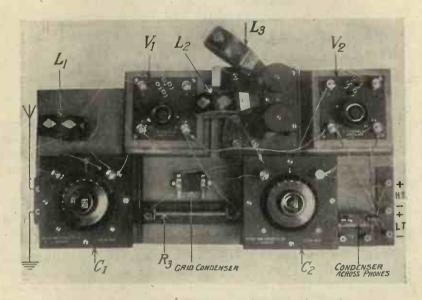
Fig. 1. Illustrating the arrangement of the two-valve receiver.
