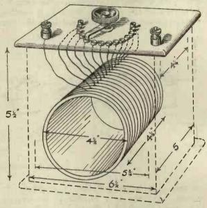
Fig. 6. The coil in position.
