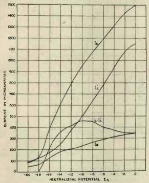
Variation in anode and collector currents I, and I. with variation of neutralising potential En.
