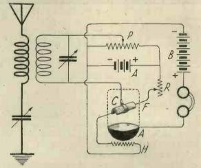
Fig. 2. Circuit of the new rectifier tube. Note the resistance in series with the filament. The current consumption is about the same as that of a standard tube.
