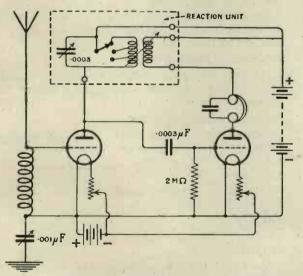
Fig. 3. Showing the connection of the coupling device.
