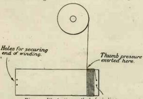
Fig. 1. Illustrating method of winding.
