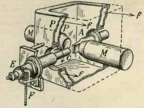
Fig. 7. A diagrammatic representation of the interior of an arc chamber.
