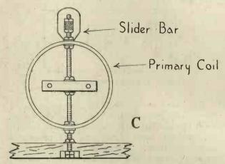
Fig. 9. Showing the position of the supports for the secondary within the primary.
