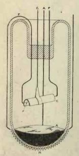
Fig. 1. Illustration of the new tube, showing internal construction. The tube itself and the resistance heating the sodium are enclosed within another glass bulb.
