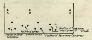
Fig. 6. Plan of the base-board.
