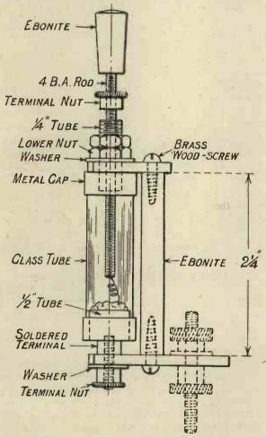
Fig. 1. General arrangement of detector.
