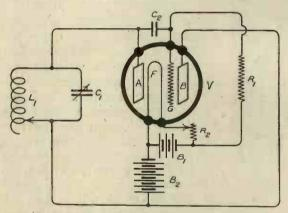
Fig. 4. The negatron employed as a generator.
