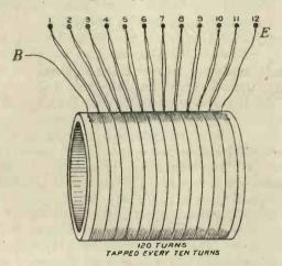
Fig. 5. Illustrating the method of winding the inductance coil with 12 tappings.
