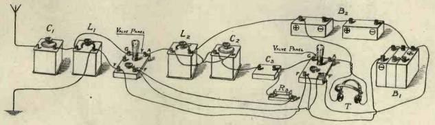
Fig. 2. Connections of the two-valve set.
