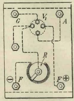
Fig. 12. Wiring of valve panel, seen from above.
