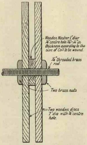
Fig. 1. Section of slab coil winder.
