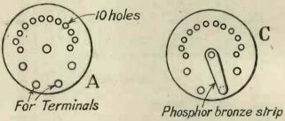
Fig. 2. Arrangement of secondary switch.
