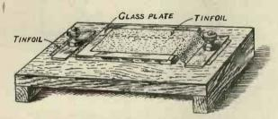
Fig. 8. Illustrating a home-made grid condenser.
