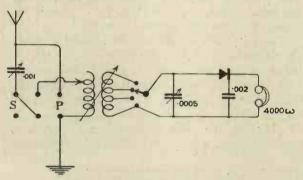
Fig. 8. The circuit of the receiver.
