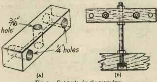
Fig. 7. Supports for the secondary.
