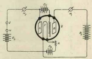
Fig. 2. A circuit for obtaining the characteristic curve of the negatron.
