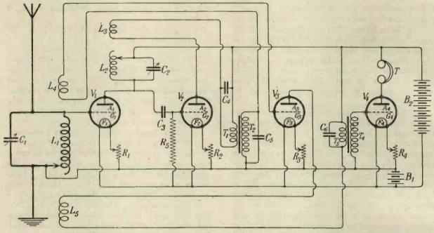
Fig. 1. The new circuit, which enables reaction effects to be produced in both aerial and anode circuits independently.
