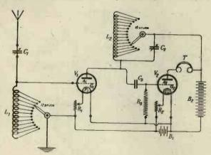
Fig. 3. Circuit of the two-valve receiver.
