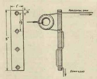
Fig. 1. Showing dimensions of the ebonite strip and its mode of attachment.
