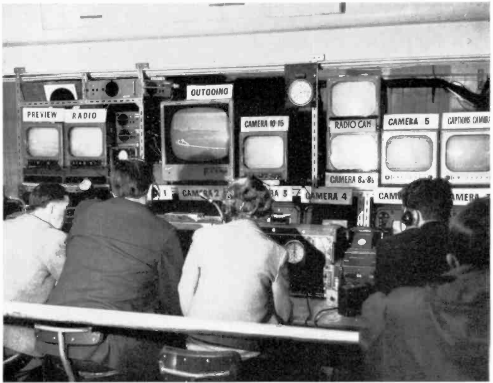
Where the sports pictures on a Grandstand location are received. To this mobile control room, are linked cameras dotted round a race course—including a light “radio camera” being carried on a TV man’s back.
