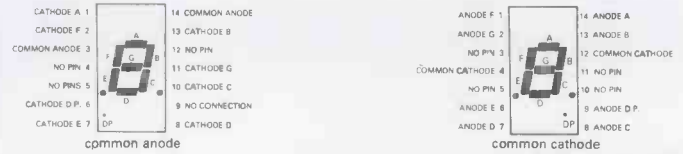
PIN CONNECTIONS (TOP VIEW)
