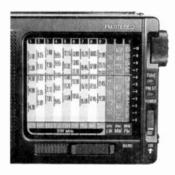
that moves a pointer across a tuning scale. Tuning is not as precise as digital tuning.
