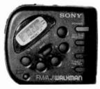
Digital personal radio with FM and MW and 10 presets. Presets are structured 5 FM and 5 MW. The presets are operated by 5 one-touch buttons. They were a little tricky to set-up, but once set, they were easy to use. Part of the problem in setting the presets and finding stations, was that the radio scans very slowly through the bands. There is a local/DX switch, but we
