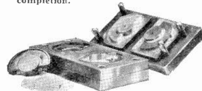
A bakelite moulding tool and powder.
