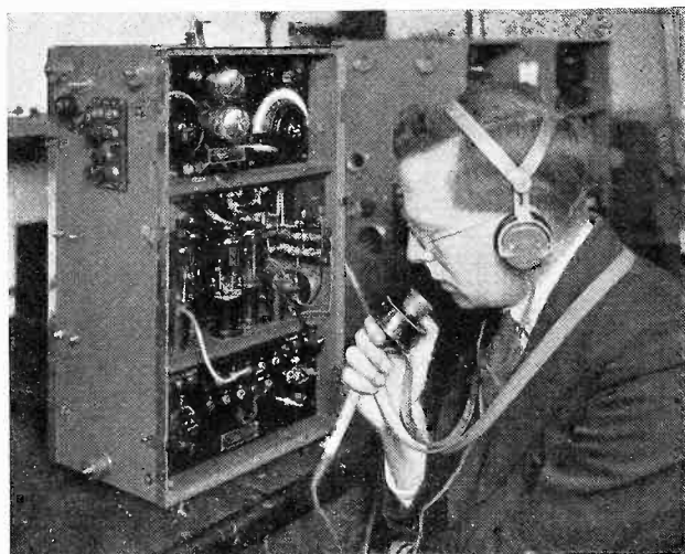
Marconi aircraft equipment Type A.D.6N undergoing final tests.
