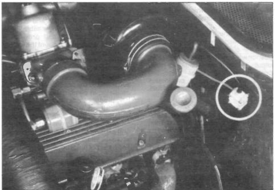
Flow transducer fitted in fuel line.
