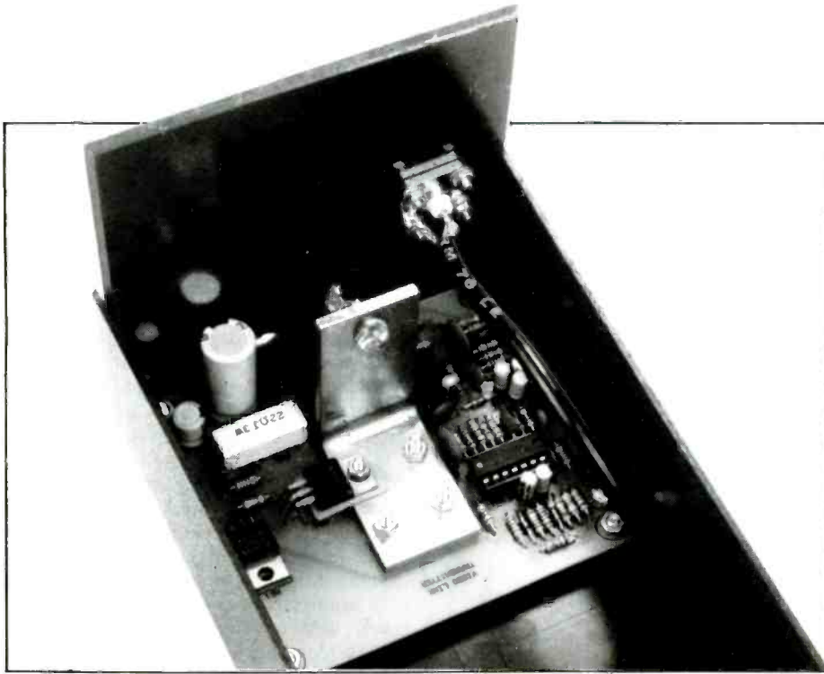
Infra-Red Video Link transmitter with top lid removed, showing internal assembly detail.
