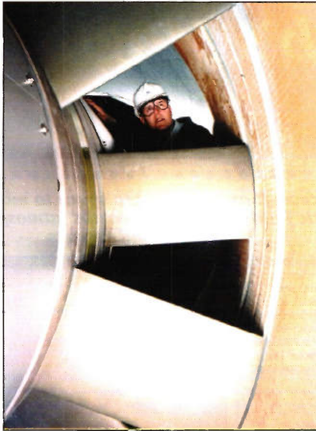
Photo 7. Detail of one of the turbine units of LIMPET 500 (Courtesy WAVEGEN)
