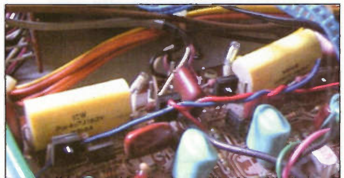
Yellow high grade polypropylene capacitors fitted to pre-amplifier.
