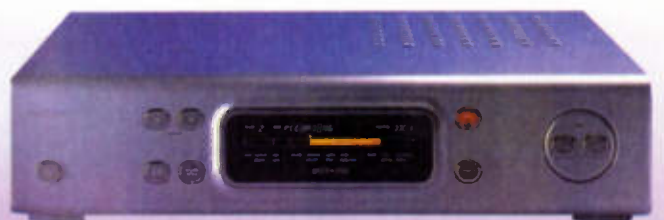
Alternatives to hard disk recording from Pioneer and Philips. These machines make use of removable, rewritable phase-change media.
