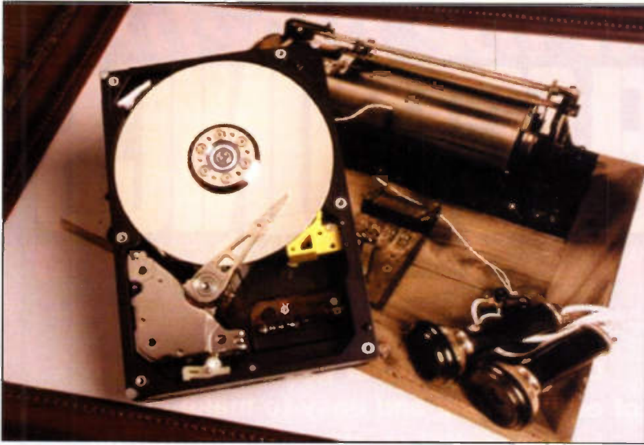
Recording set-top boxes would probably be based around high-capacity PC drives, like this 25Gb IBM model
