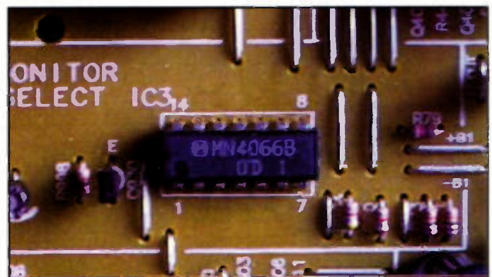
4066 IC used as a monitor/input select in a typical 3-head tape deck.
