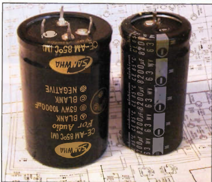
The replacement psu capacitors are different in size to the originals.
