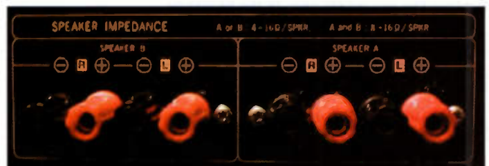
Power amplifier with new speaker sockets.
