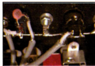
Close-up view of S-Video socket and composite/S-Video switch wiring
