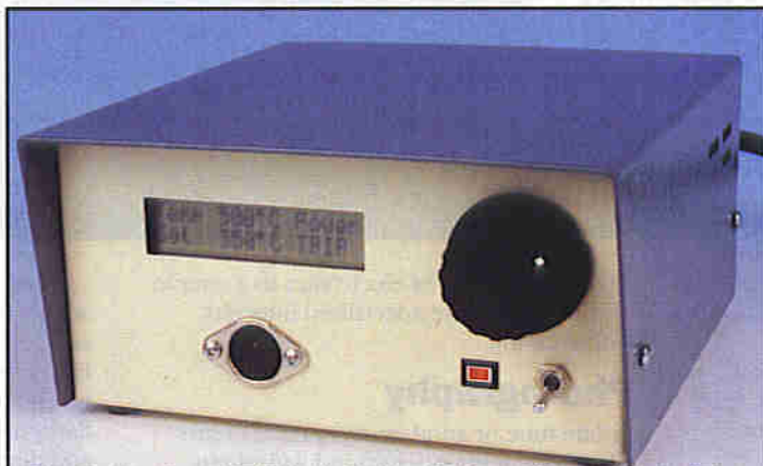
The display shows 'TRIP' to indicate a fault condition exists, in this case, caused by the soldering iron being disconnected from the unit.
