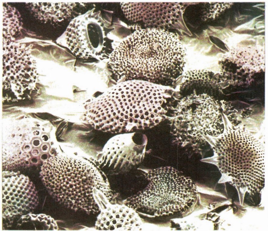
Photo 1. Typical image obtained of Diatoms (fossil algae) at 200\times magnification using a Leica Stereoscan 440 Scanning Electron Microscope. (Courtesy, Leica, Cambridge, UK.)
