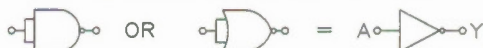
Figure 12. Any NAND or NOR gate can be used as an inverting buffer element.
