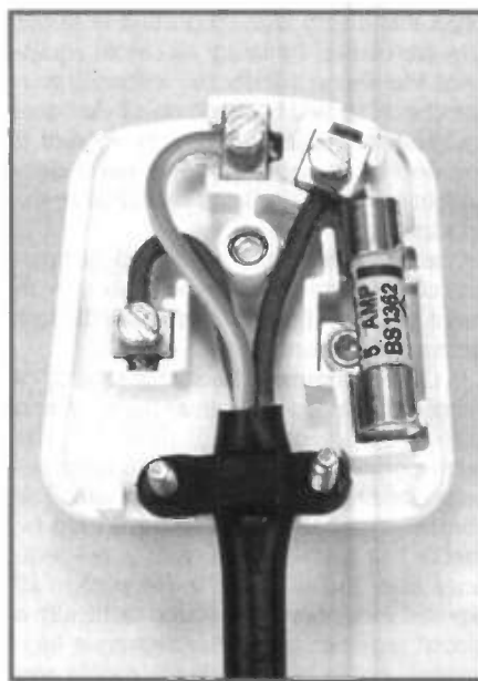
Above: Photo 8. Correctly wired mains plug. Below: Figure 9. Example of Class II construction.
