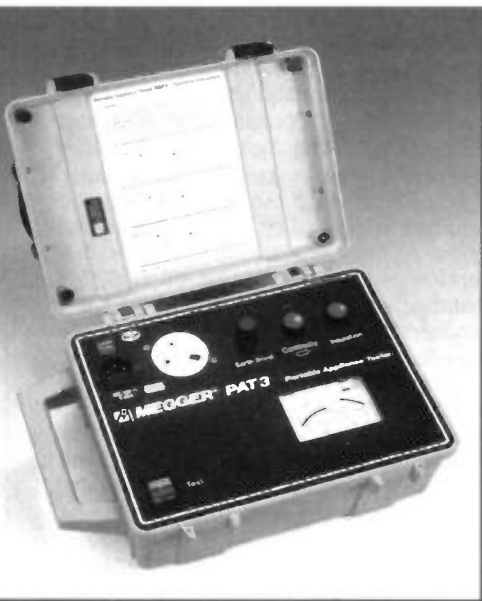
Photo 9. Portable Appliance Tester (PAT), used to check for earthing continuity between appliance and plug, live/neutral shorting to case, and plug/appliance fuse testing.
