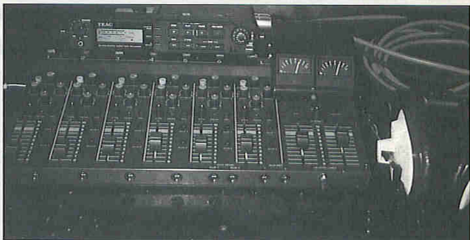
Photo 3. Compact 'budget' location recording equipment system using battery powered mixer and DAT recorder.
