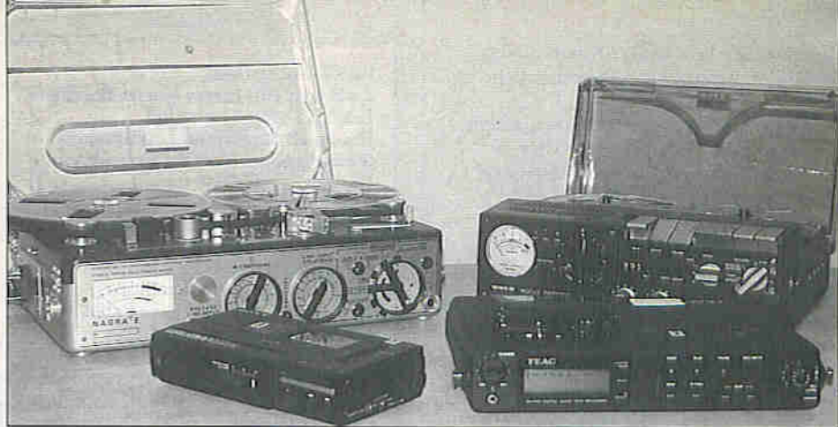
Photo 2. Professional portable recorders. Left to right (rear) Nagra E, Uher 4000, (front) Sony WM D6C cassette recorder, Teac DA-P20 DAT recorder.
