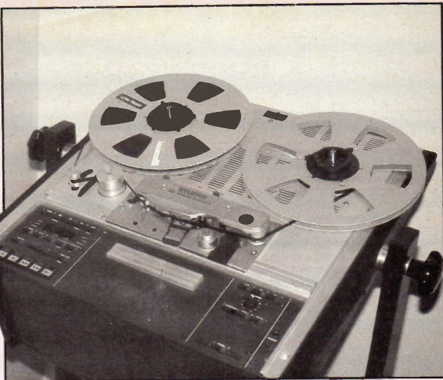
Studer A807 professional recorder - note absence of any superfluous user controls.
