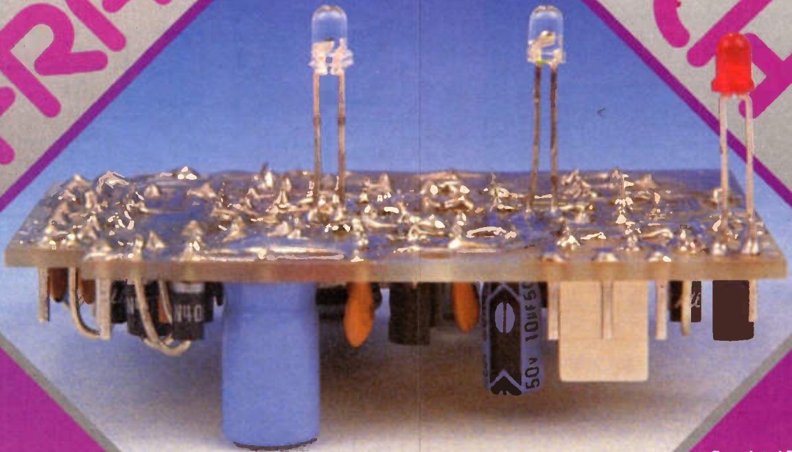
Completed PCB – track side, showing how LD1, IR1 and PD1 are mounted.
