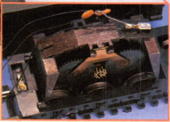
Bottom photograph and inset photographs show fitting of the receiver module to a locomotive with a Ringfield type motor.
