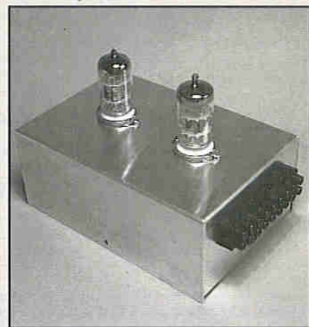
Completed chassis with valves in place.
