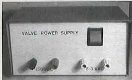
The completed power supply unit (note prototype shows 4mm terminal posts, it is strongly recommended that 4mm 'touch proof' sockets are used instead for reasons of safety).
