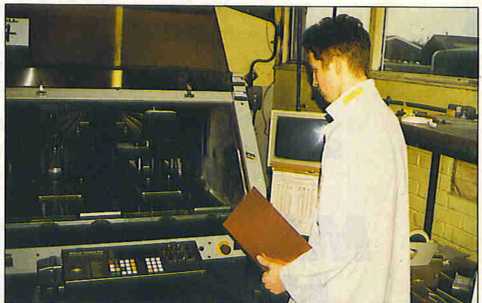
Photo 1. One of the five CNC drilling/routing machines that PMS uses. Just above the control panel of this Wessel CompacTrol machine, you can see the tool bay; the machine can be programmed to change bits automatically.
