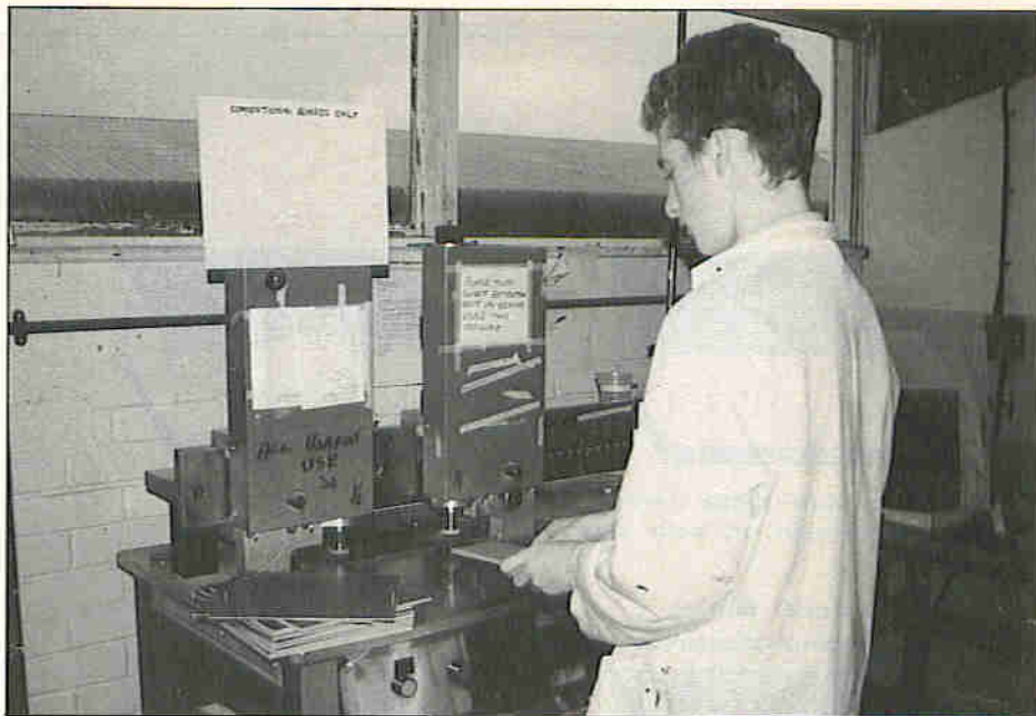
Photo 2. Here we see the Bohan pinning machine, which is used to drill the alignment reference holes.
