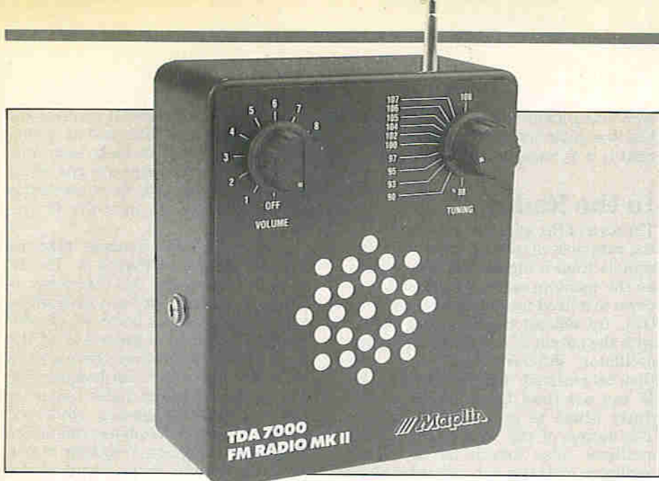
The Maplin Mk.2 FM Radio, based around the TDA7000 IC. Details on this set can be found in Issue 27 (June/August 1988) of 'Electronics'.
