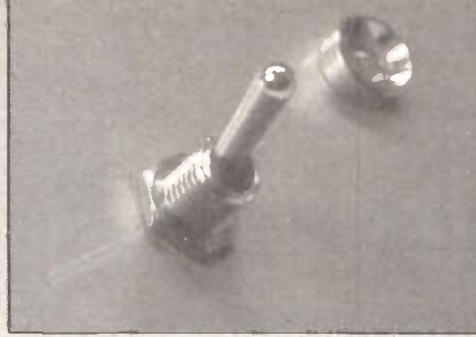
Photo 5. (above) A view of a front panel showing how not to fit an on-off switch. In this instance, the second securing nut (which normally fits behind the panel) has been omitted, leaving too much threaded switch shaft on display.
