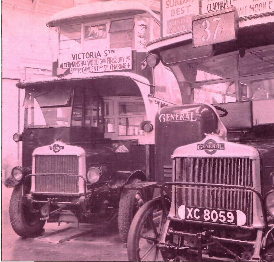
Left: Rapid evolution in the 1920's. 'K' type bus (right), built in 1920, has an open top and cab, and solid tyres. 'NS' type bus (left), built in 1927, has an enclosed top deck and cab, and pneumatic tyres.
