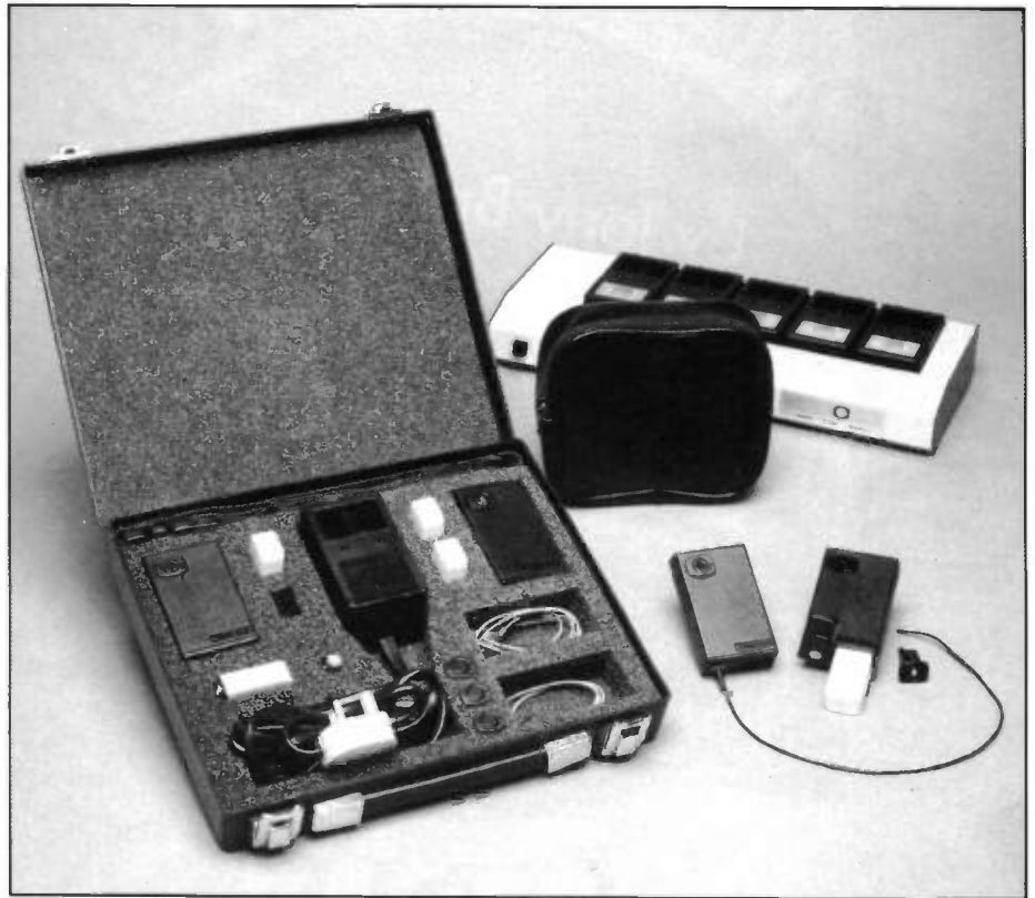
Photo 6. A Radio microphone and receiver system designed for the hearing impaired.
