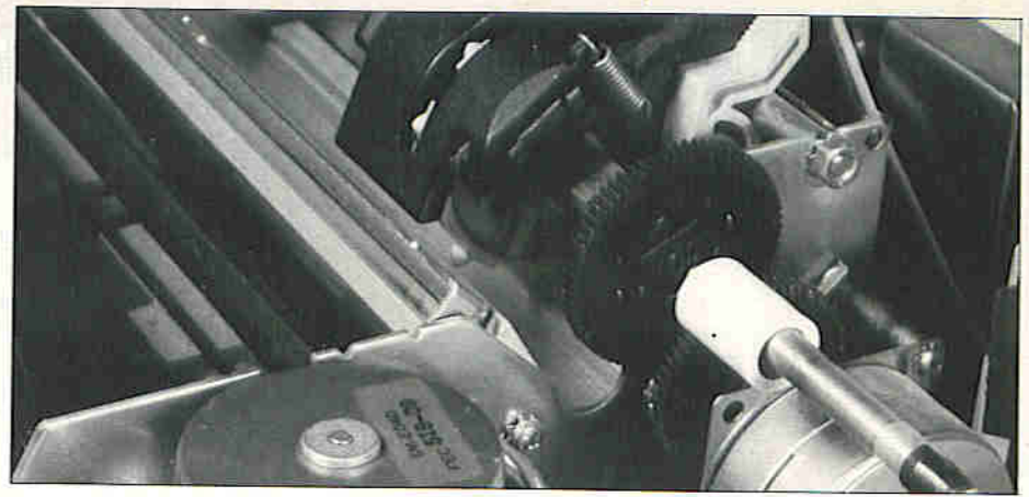
Photo 1. Stepper motors used in Epson printer. Left motor drives head via toothed belt; right motor drives platen via gearing.
