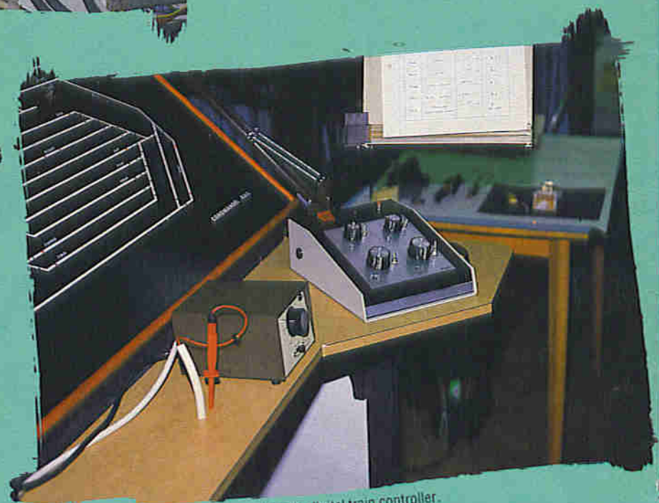
Photo 5. 'Mimic' control panel and Maplin digital train controller.
