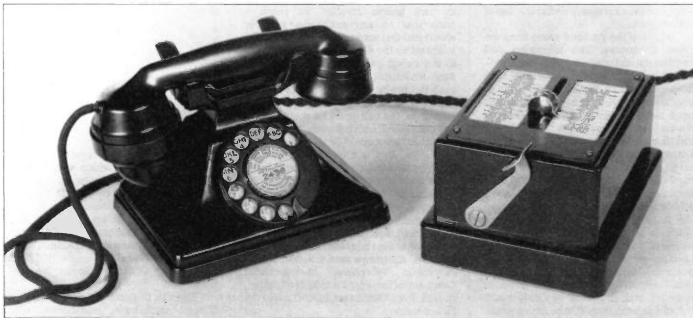
Photo 1. The 162 telephone illustrating a useful feature – a clockwork autodialler.
