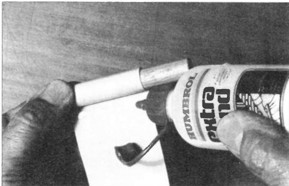
Photo 1. A cheap and easy way of making coil formers – winding thin card strips onto a suitable former and glueing the layers with PVA glue.
