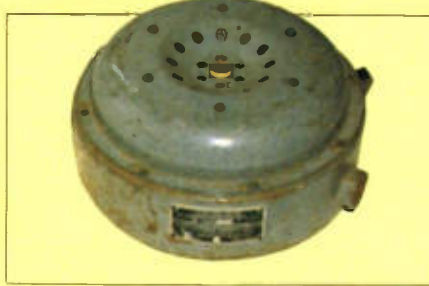
Photo 1a. Loudspeaker at war. A 160mm driver with a bakelised fabric cone was made by RCA for use in this US Navy direct-radiator outdoor loudspeaker. An inbuilt transformer allowed matching to both low-impedance and 'constant voltage' amplifiers.
