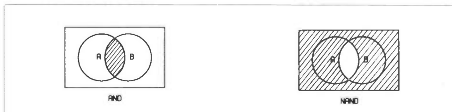
Figure 22. Venn diagrams for AND and NAND.
