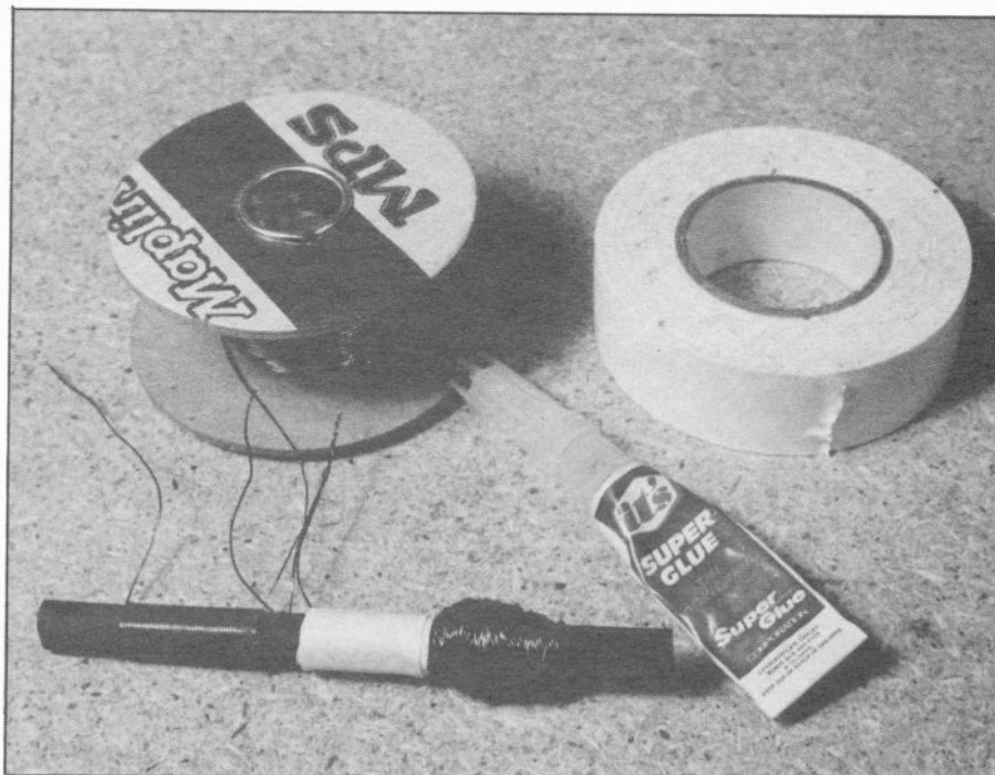
Photo 3. Compare the neatness of the medium wave coil (secured with glue) and the 'scramble wound' long wave coil (secured with a piece of PVC tape).
