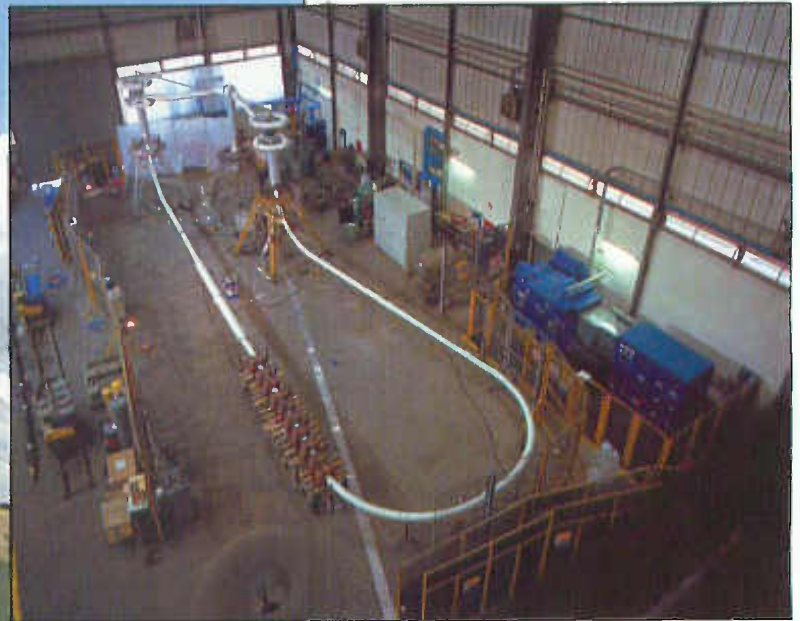
Figure 11. A length of finished superconductor power transmission cable, undergoing test.
