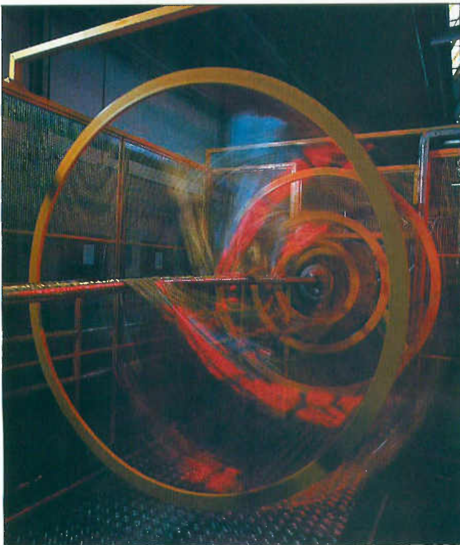
Figure 12. Applying the mylar insulation over the cryostat during cable manufacture.
