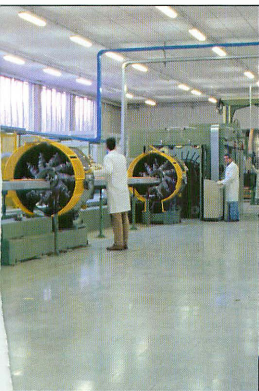
Figure 13. Pirelli's first pilot line circa 1996, dedicated to HTS conductor 'stranding'
