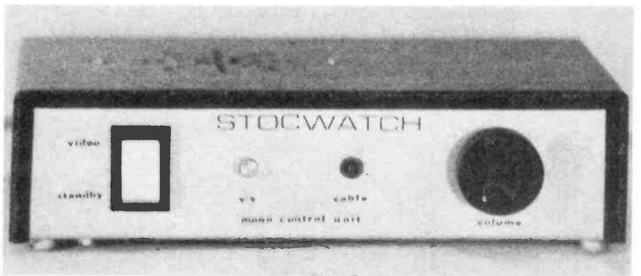
Figure 13. A camera control unit and modulator using the UM1286.
