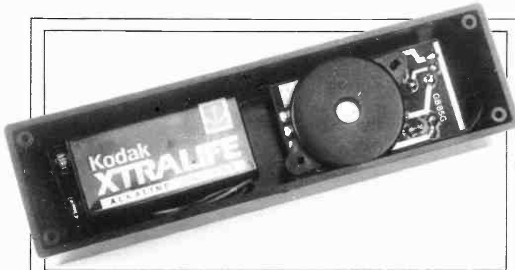
Inside view of the Live-Wire Detector prior to fitting the back panel.
