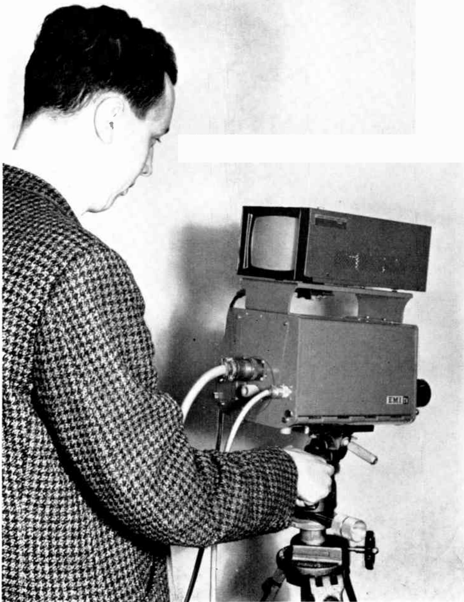
Camera 'B' of EMI's Type 9 concept. This is a self-contained camera with only a single cable linking to the power unit. Ingenious little electronic viewfinder is optional.
