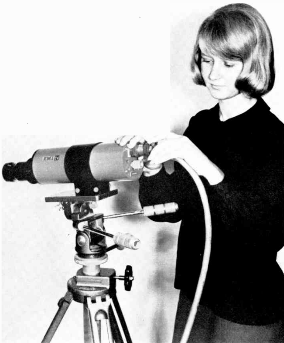
Camera 'A' of the startling new EMI Type 9 CCTP concept. This unit is only 9.5-cm in diameter, is solid-state. A 32-way cable connects with the modular control and remote-control units.
