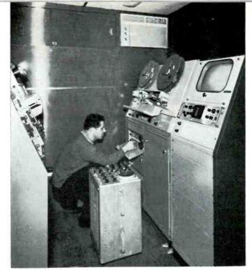
Interior view of recording room showing one of the two Ampex fully transistorised audio video tape recording units operated by Intertel (VTR Services) Ltd and mounted in a Luton body on a Ford D 800 chassis.
