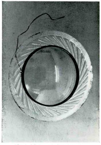
Melinex 1 mil diaphragm and coil unit of new STC tweeter.
