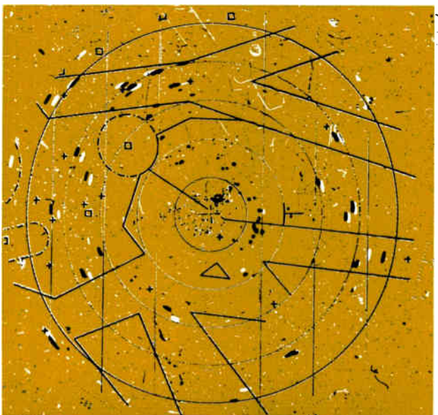
Fig. 2. These two radar pictures of the Ash Marconi S264 were taken at the London ATCC. The first (a) was taken when normal MTI was in operation, while the second (b) was taken thirty seconds later during SMTI. The SMTI clearly shows a number of additional returns from aircraft which were not visible with MTI. The bottom diagram shows a and b superimposed. (Crown copyright photographs)
