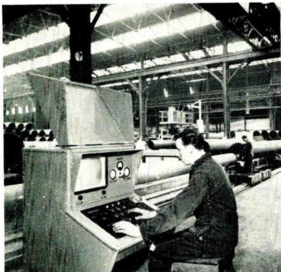
Stewarts and Lloyds' British Tube Works in Birmingham is using c.c.t.v. to assist the internal electric-fusion welding of large diameter pipes (left); the operator controls the welding by referring to the picture monitor on his control console. On the right, the cover from the head of a quasi-arc boom-welding machine has been removed showing the c.c.t.v. camera that is used for accurately guiding the welding electrodes
