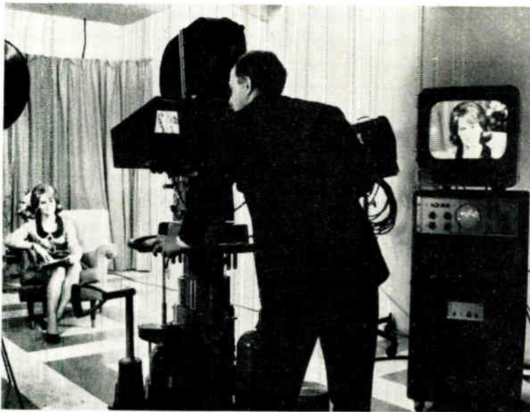
The Add-a-Vision is here shown mounted on a Mitchell BNC 35-mm camera. The picture on the 7-in. electronic viewfinder is repeated on the large screen monitor above the control console
