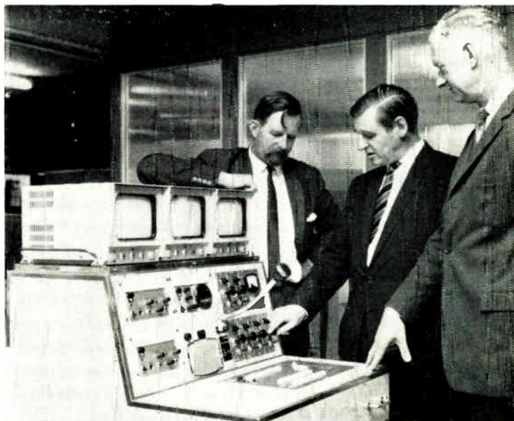
A complete mobile television unit, designed to show classroom techniques in teacher-training colleges, but having obvious applications in industrial training and communication as well, has been produced by Pelo Scott Ltd. Its console is a complete mixer/control unit (fitted for two live television channels, v.t.r. and sound) and its three main component parts can be carried by two men
