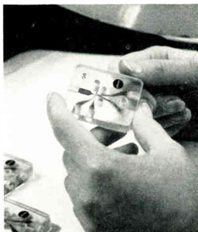
Fig. 2. (a) (left) an OR/NOR fluid-logic element, one of four fluidic devices now being marketed by the Plessey Components Group; (b) (right) the Plessey shift register stage element, which can perform a number of operations besides counting
