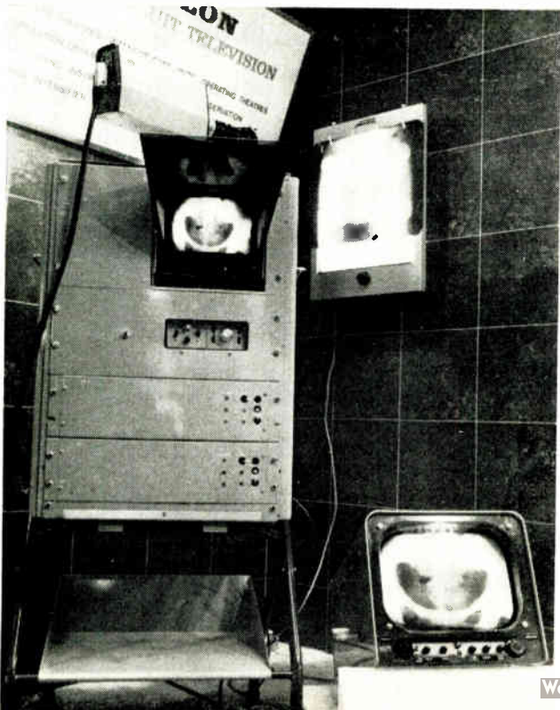
Closed-circuit television applications in the medical field were demonstrated by Epsilon Industries, who showed how the quality required for interpreting X-ray plates could be maintained by using their high-definition c.c.t.v. cameras and monitors (81). In such areas as operating theatres, only small camera heads need be used, which can be equipped with remotely-controlled zoom lenses and closed-up attachments and then fitted to the theatre lamp. Their c.c.t.v. equipment can also be used with a wide range of endoscopes, as well as for ward surveillance and hospital communications
