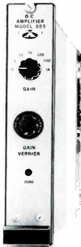
Model 885-235 D.C. Amplifiers Gain Range : 3 to 3000 Input Resistance : 100 Megohms Bandwidth : d.c. to 10 kc/s Output : 10 volts at \pm 100\text{mA} Drift : 1\mu\text{V} for 40 hours Temp Coeff : 0.2\mu\text{V}/^\circ\text{F} Noise : 2\mu\text{V rms}
