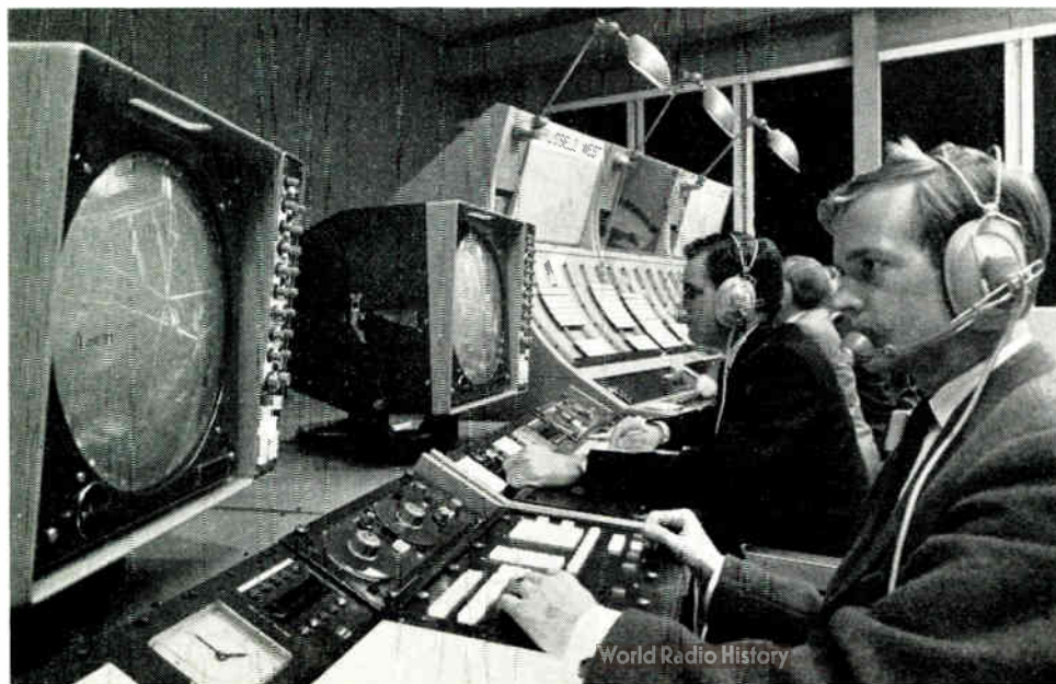
Here can be seen an air-traffic controller's console. The radar screen depicts the positions of each of the simulated aircraft, any one of which can be marked using a rolling-ball controlled marker, and can also display a video map. Each time the controller requires information on an aircraft or requires an aircraft to alter course, he will contact the pilot-operator controlling that aircraft and pass the message over the telephone system
