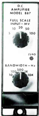
Model 887-115 Dual Output Differential Amplifier Gain Range : 1 to 5000 Input Resistance : 25 Megohms Drift : 2\mu\text{V} for 40 hours Temp Coeff : 0.5\mu\text{V}/^\circ\text{F} Noise : 1 to 7 \mu\text{V rms} (depending on bandwidth) Output A : 10\text{V} @ \pm 100\text{mA} Bandwidth A : d.c. to 60 kc/s Output B : 10\text{V} @ \pm 10\text{mA} Bandwidth B : front panel selected 10 c/s, 100 c/s, 1000 c/s & 10,000 c/s
