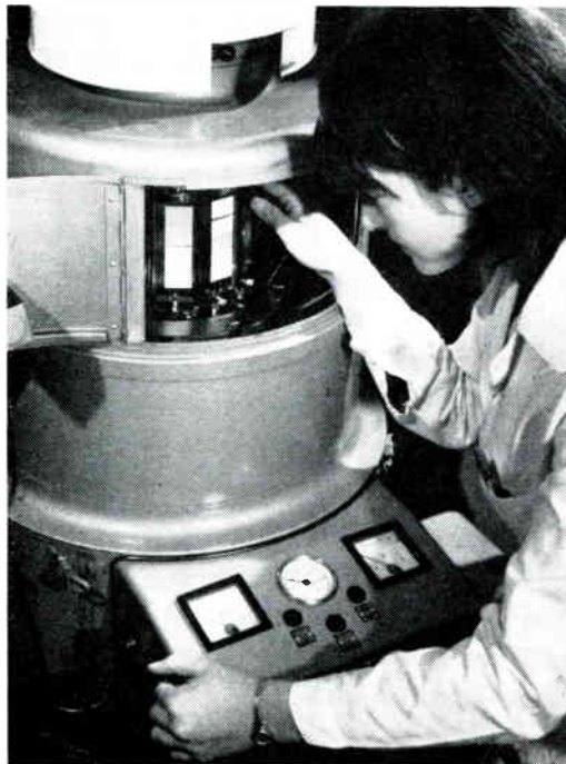
Here the equipment is being set up for a test period lasting 1,600 hrs—equivalent to about two years' exposure to sunlight
