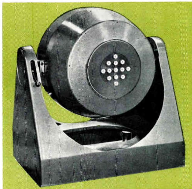
Fig. 5. The vibrator shown, a Pye-Ling shaker model V1007, is air cooled and has a force rating of 1,800 lb thrust and a bare-table acceleration of 90 g
