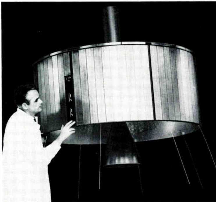
This picture of the INTELSAT satellite shows the solar cells around the outer shell, the motor at the bottom of the structure, and the microwave aerial at the top
