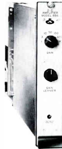
Model 886-101 D.C. Amplifiers Gain Range : 1 to 3000 Input Resistance : 100 Megohms Bandwidth : d.c. to 50 kc/s Output : 10 volts at \pm 100\text{mA} Drift : 1\mu\text{V} for 40 hours Temp Coeff : 0.2\mu\text{V}/^\circ\text{F} Noise : 2\mu\text{V rms}
