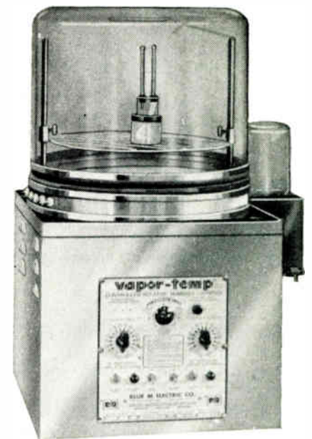
▲ Shown here is one of the test chambers featured by Blue M Electric Co. Known as the 'Vapor-Temp', it is a controlled temperature and relative humidity chamber for testing electronic components and laboratory specimens under controlled conditions. The unit consists of a base section containing the controls, motor and blower, water reservoir, cooling coil and heating elements. The chamber is formed by an inverted Pyrex jar, 14-in. high \times 16-in. diameter
