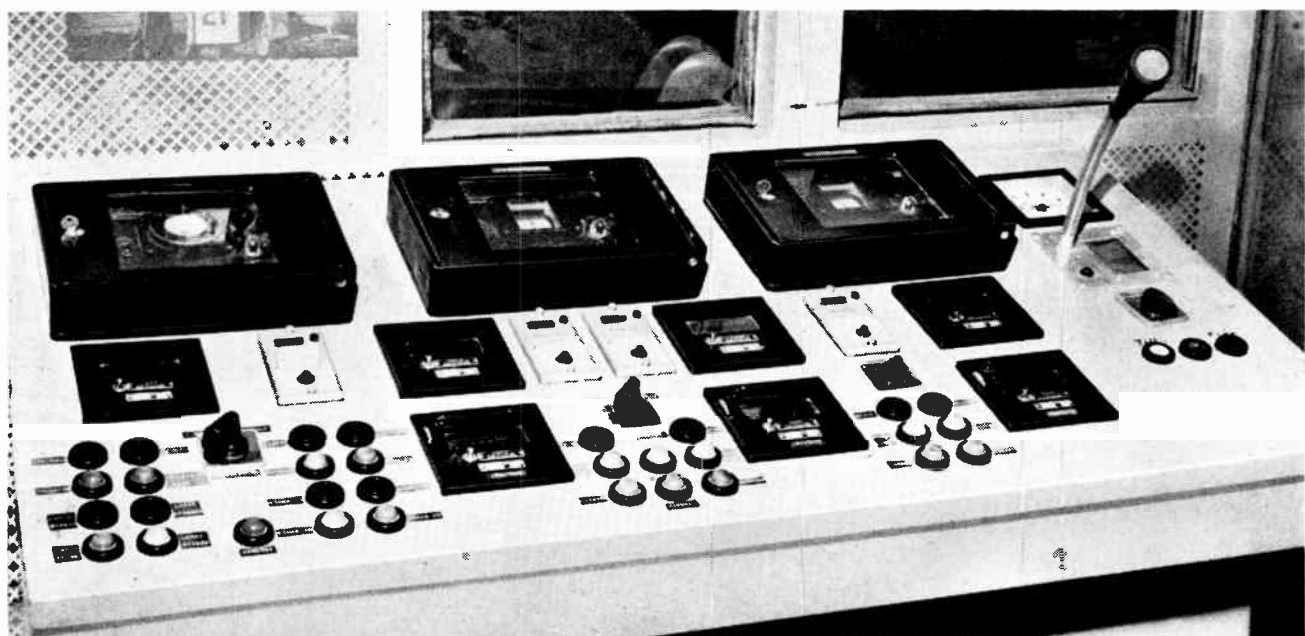
Additions feed control desk, part of the Rank Flotronic continuous-weighing equipment in the Norrbottens steel mill. The picture shows controls for the batch-weighing and hopper-weighing systems installed, and the digital printouts for both
