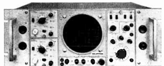
* CX 1447 A rack-mounting case is available as an alternative for use in standard 19" racks. Side panel design permits simple signal connections from rear of instrument.
