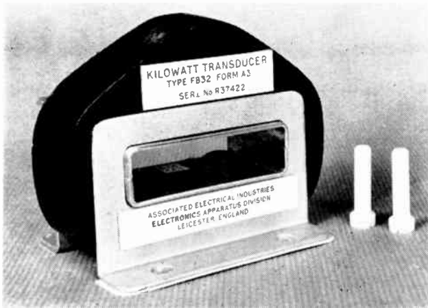
Fig. 5 (Left). Kilowatt transducer incorporating a Hall effect device
