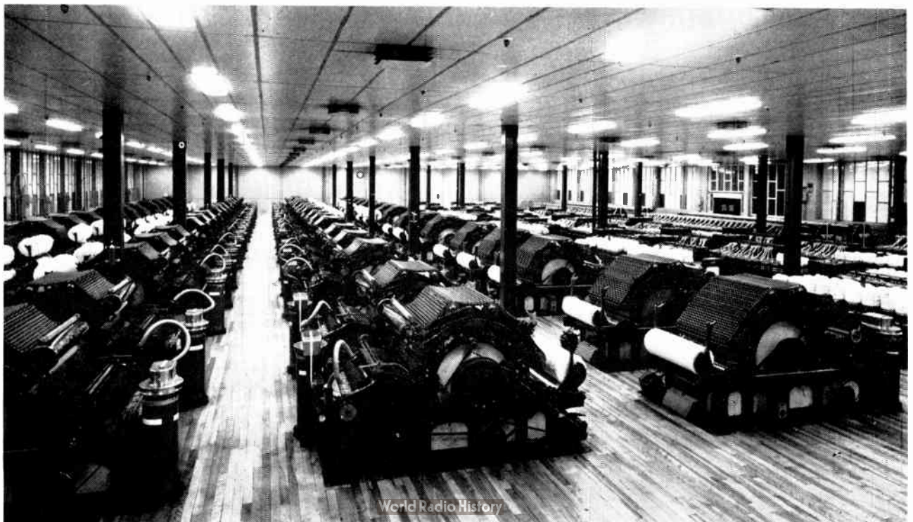
Fig. 1. An installation of Platts cotton cards showing the roll of feed sheet at the input and the peeled off web condensed into a rope-like sliver at the output
