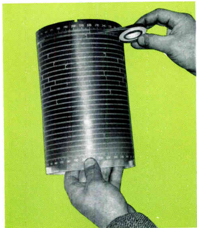
Applying a tape strip to a programme drum
