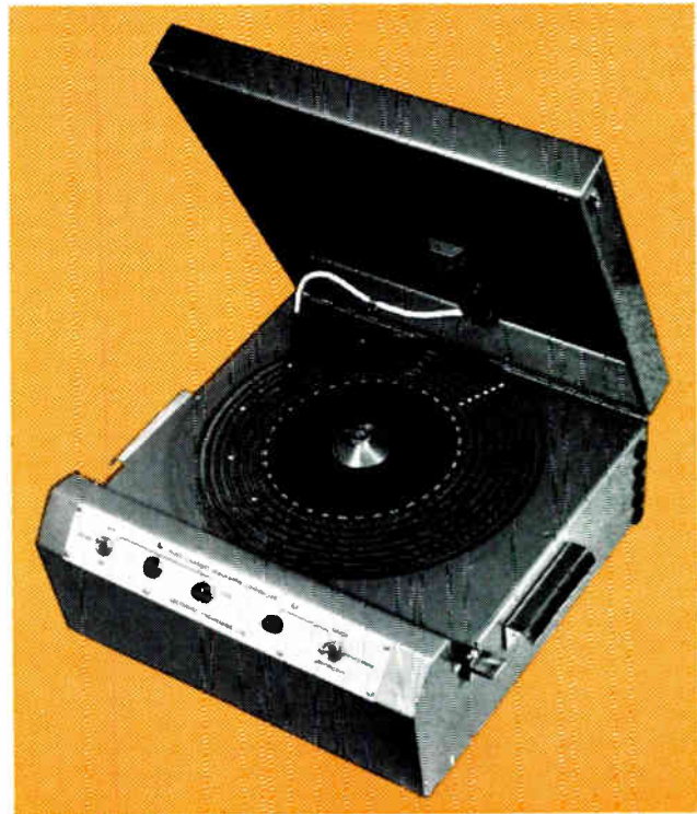
Programme controller using a disc with annular rings
