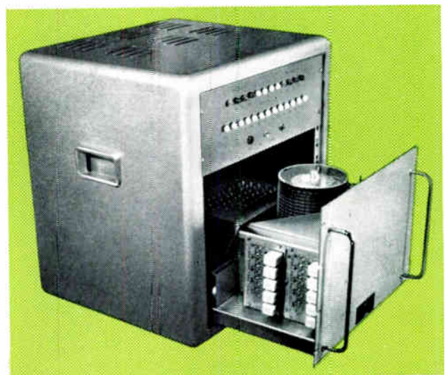
Complete controller with a taped drum inserted
