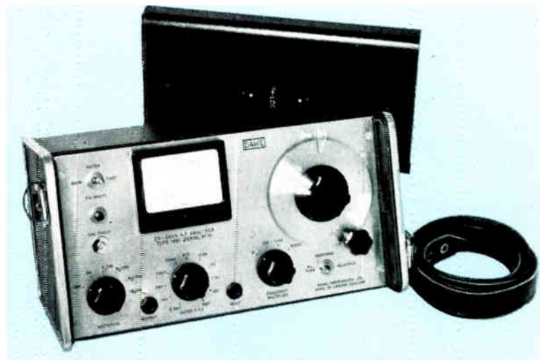
A typical portable a.f. analyser complete with self-contained power supply
