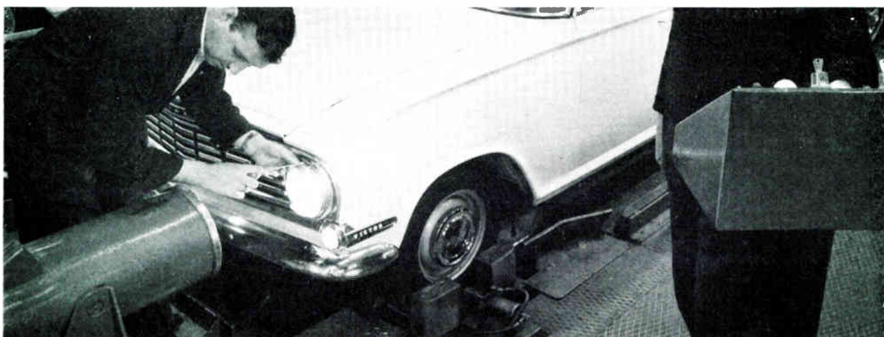
A car stands on the apparatus and at the same time the headlights are adjusted
