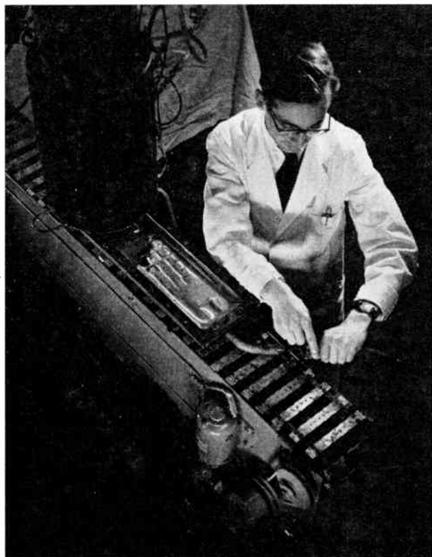
RADIATION TESTING OF INSULATED MATERIALS —When insulated materials are liable to be exposed to nuclear radiation during service it is necessary to have prior knowledge of the amount of radiation which they will withstand before they become unsuitable for further use. In the research organization of BICC materials are subjected to electron bombardment from a 2-MeV particle accelerator while enclosed in a specially-designed vacuum cell
