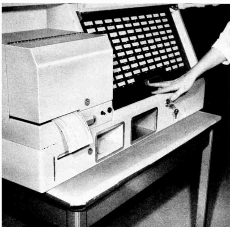
Plates pushed into station with record voucher. 'Start' button is pressed
