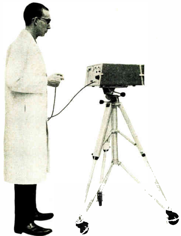
Portable Fexitron machine capable of radiographing all parts of the human anatomy
