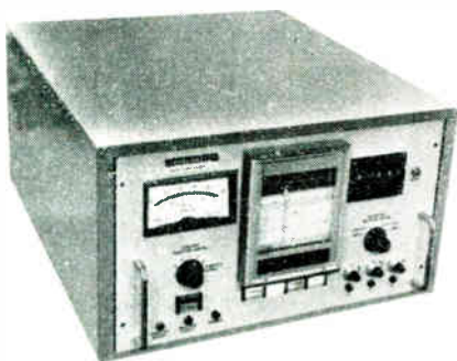
Honeywell's new on-line mass flow computer introduced at the show. It is built from standard plug-in modules and accepts input signals from a variety of devices. The accuracy is \pm 0.5\% over the temperature range 30 F to 120 F (48)
