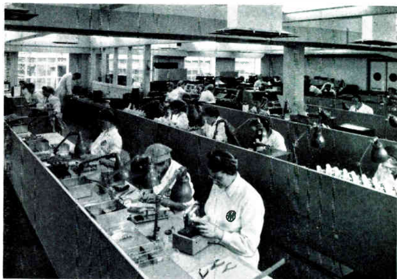
Fig. 2. Air-conditioned zone in which movement assembly and final testing are carried out
