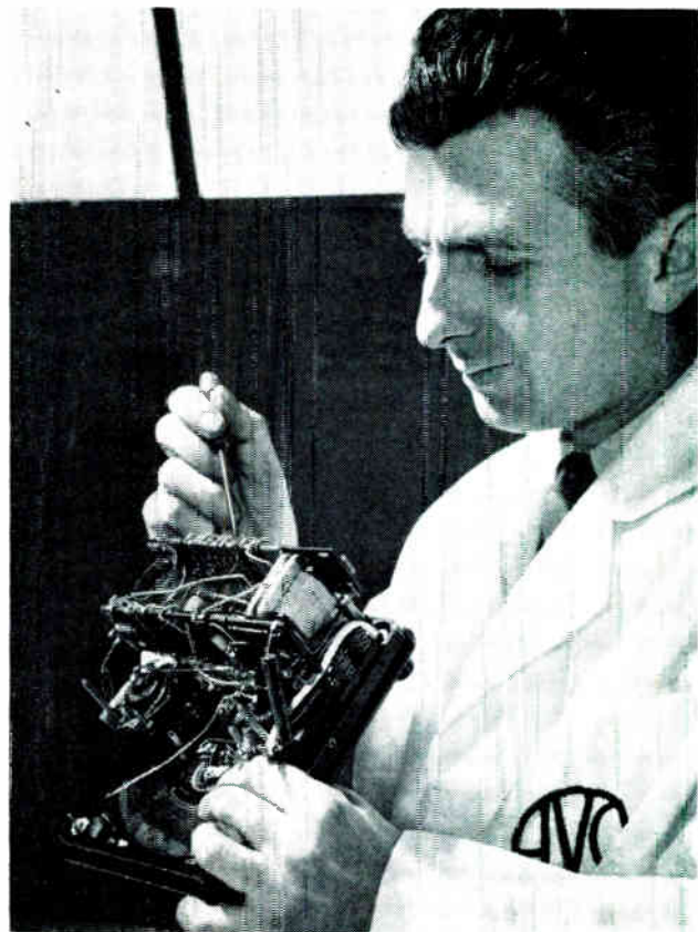
Inspecting vantage-dropping resistor panel
