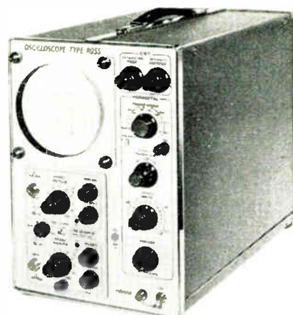
(Above) One of the four low-cost oscilloscopes introduced at the I.E.A. by Roband. Each unit uses a 5-in. c.r.t. The instruments are designated R050, R051, R055 (illustrated here) and R0501. They range from a wideband precision unit to a general-purpose servicing 'scope (78)
