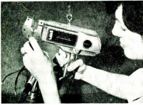
A portable power-operated crimping tool which was demonstrated by Plessey-U.K. Compressed-air driven, this UNerimp is capable of one-hand or foot-pedal operation and makes square-form crimps on any size of wire or contact up to 12 a.w.g. (88)
