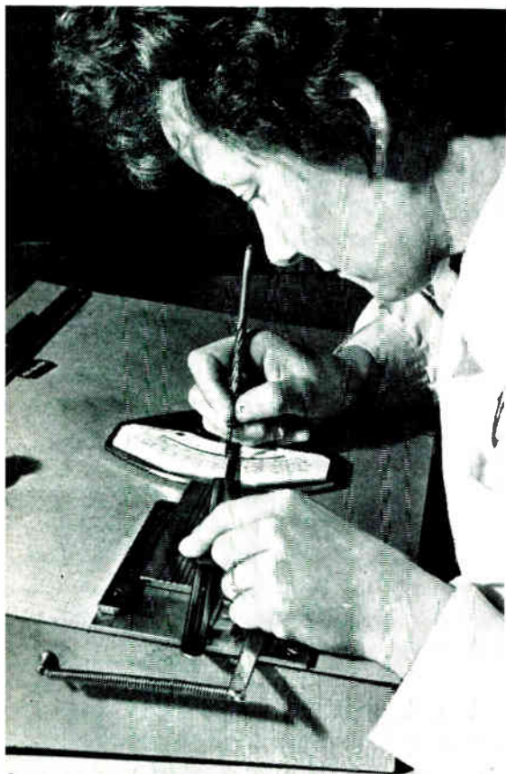
Fig. 4. Hand lining a scale plate
