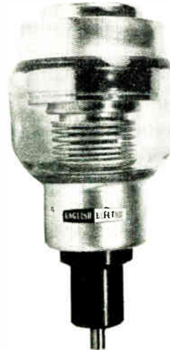
(Above) This Colvern 'Dialpot' received much attention. It is a 10-turn helical potentiometer with an integral clock type dial. 100 divisions on the dial give 1,000 settings over the 10 ten turns. There are 3-W units available in the resistance range 100 \Omega to 100 k \Omega ; standard linearity is \pm 0.25\% (94)
