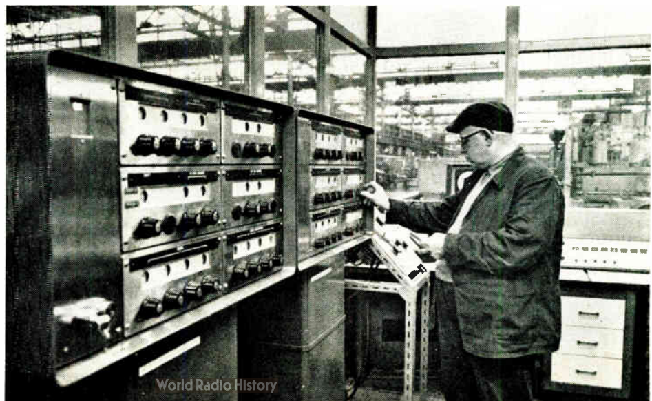
An operator feeds instructions into an ARCH computing system supplied by Elliott-Automation to the Velindre tin-plate works of the Steel Company of Wales. This is one of two identical ARCH computing systems which S.C.O.W. are using for 'on-line' quality control of high speed continuous tin strip production, the other being in operation at their Trostre works
