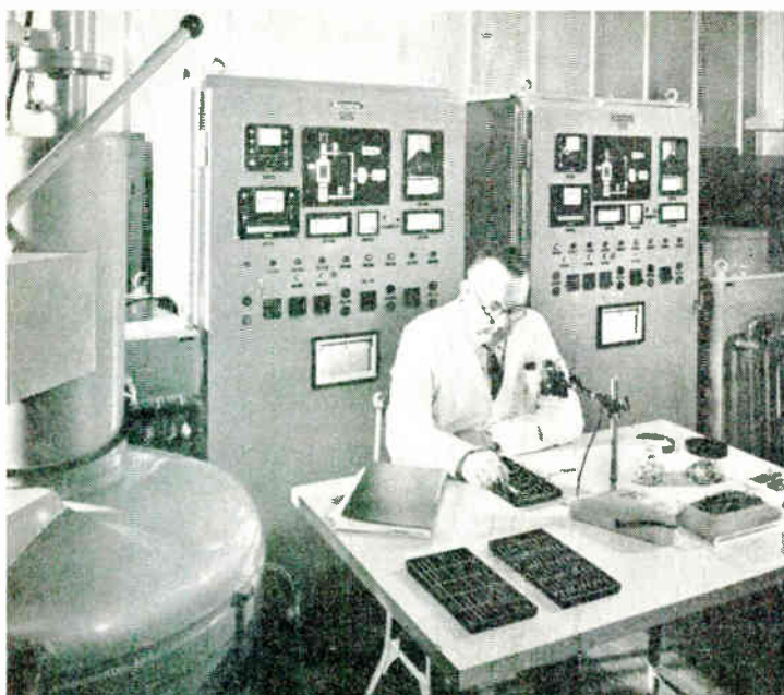
Fig. 5 Twin semi-automatic furnaces for sintering tantalum slugs
