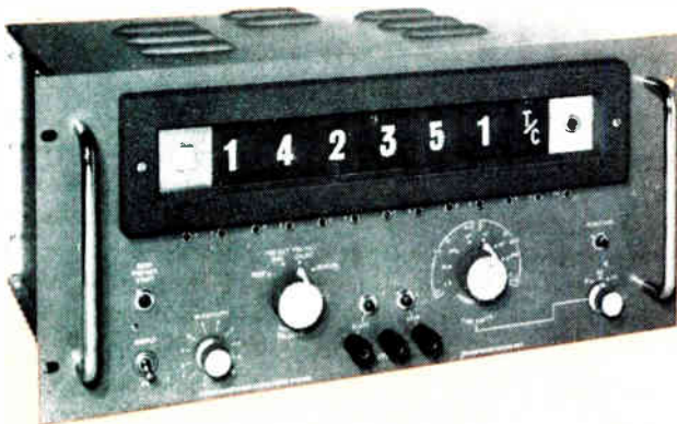
Fig. 11. Inexpensive nuclear counter
