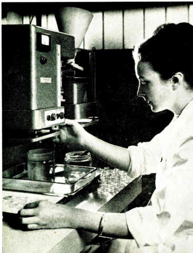
Fig. 3 Electronic dispenser for the tantalum and phosphorous powder
