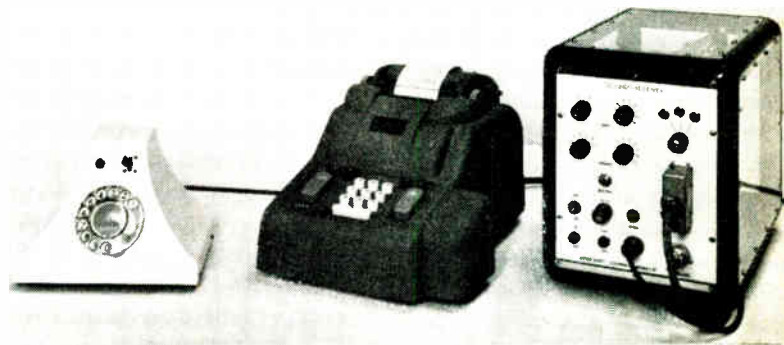
A basic Teledigit system consisting of (left to right): transmitter, Addo-X 7-digit printer, and receiver unit
