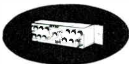
Fig. 4. (Above) Multi-indicator comprising ten sheets of Perspex each carrying a numeral. The sheets are edge lit by separate lamps (K.G.M. Electronics Ltd.)
