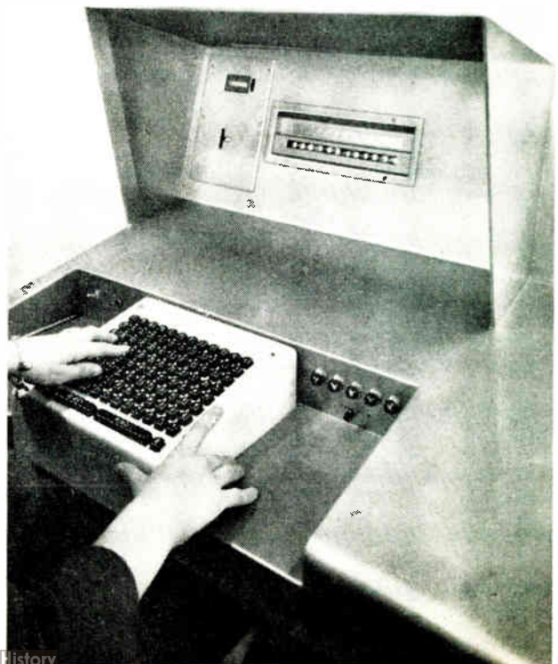
Fig. 3. The tape is perforated by an operator who sets up on a keyboard the numbers appearing projected on a screen from the master chart
