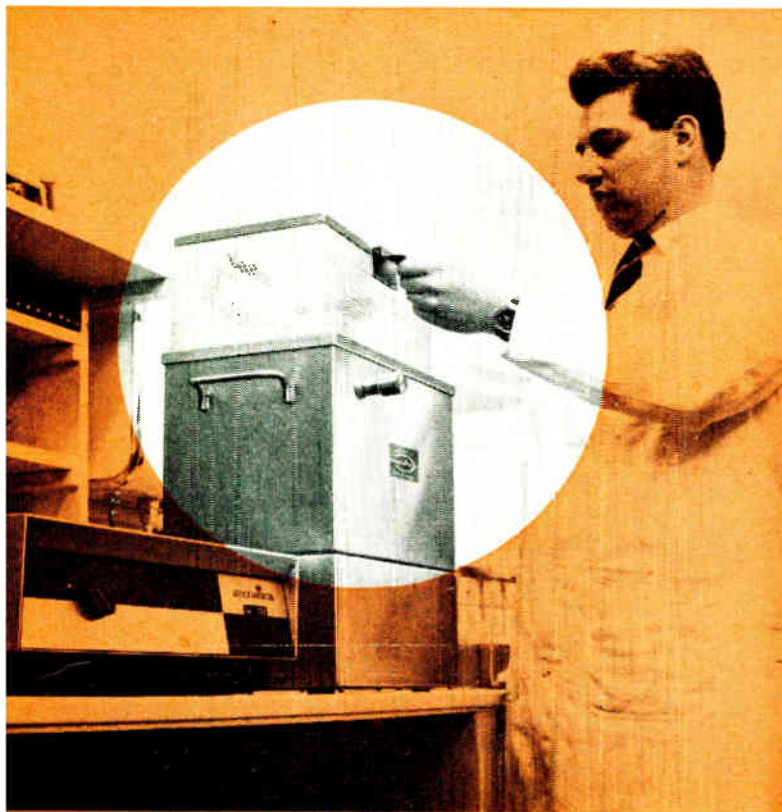
Ultrasonic cleaning bath being loaded with work in basket
