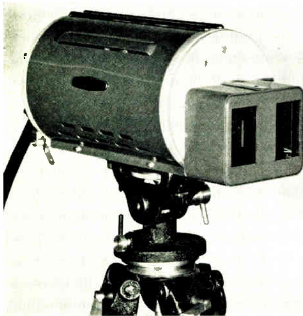
Pye television camera fitted with mirror system for three-dimensional pictures
