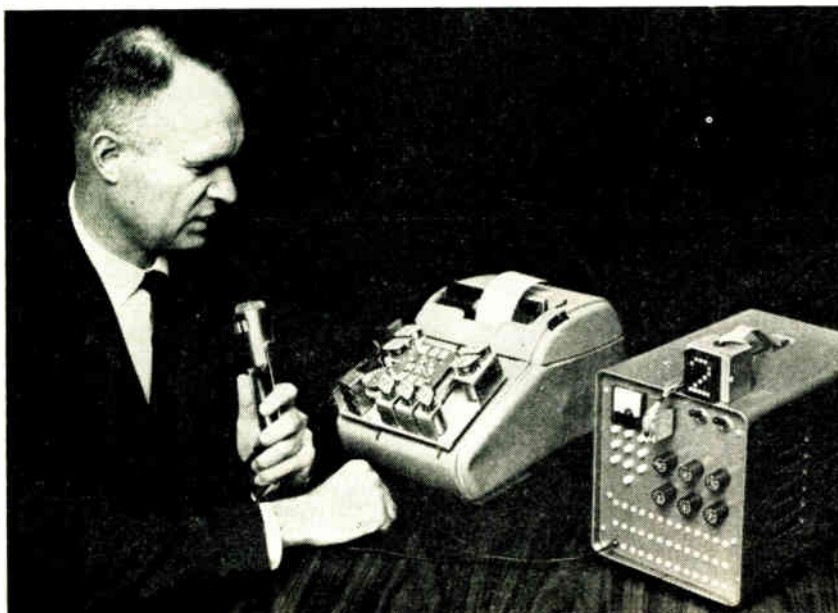
The picture shows the demonstrator speaking into a microphone connected to the apparatus on the right which operates the adding machine in the middle
