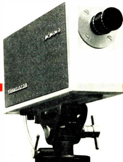
Ekco C 416 television camera for a 625-line standard. Completely transistorized and needing only a 200-250 V a.c. supply, it provides an output suitable for direct connection to a domestic 625-line receiver. A remote control of sensitivity can be fitted
