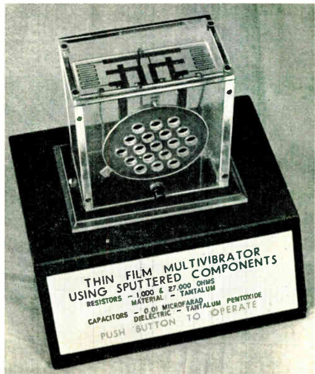
Fig. 3.—Demonstration model of multivibrator [Crown copyright]
