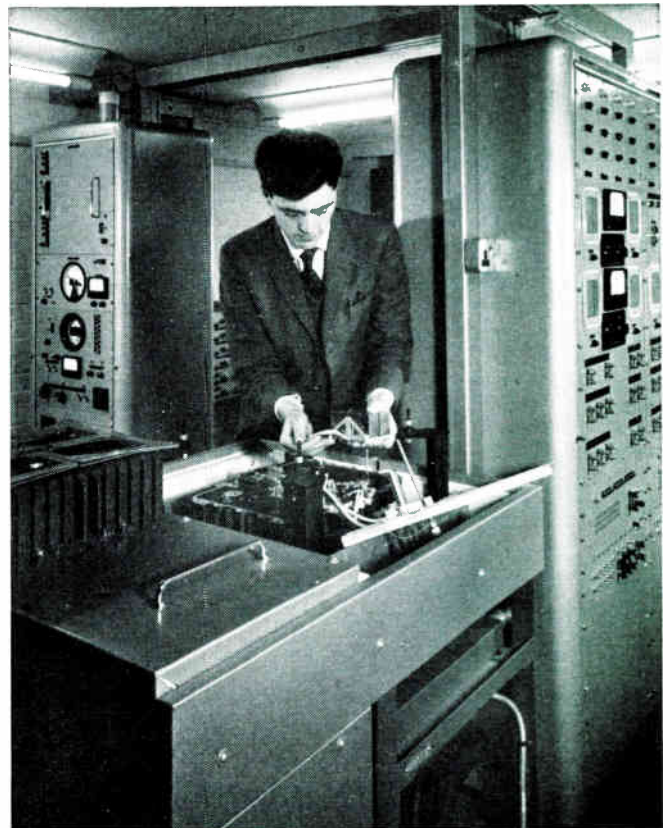
Part of the equipment for the testing of the digital integrators. The integrator is being placed in a vibrator prior to testing
