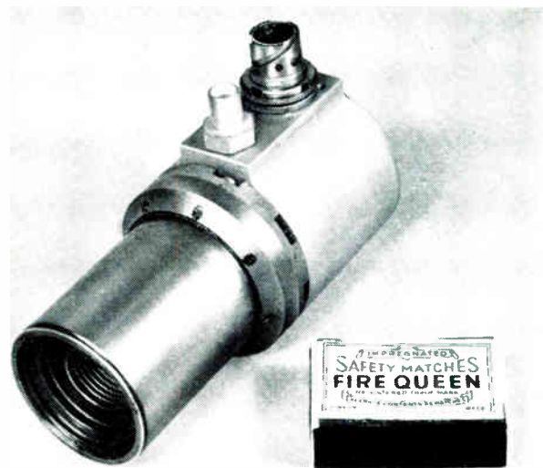
Photograph of pressure transducer
