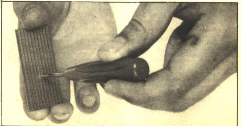
Using the special tool to cut Veroboard tracks. A drill bit is as useful
