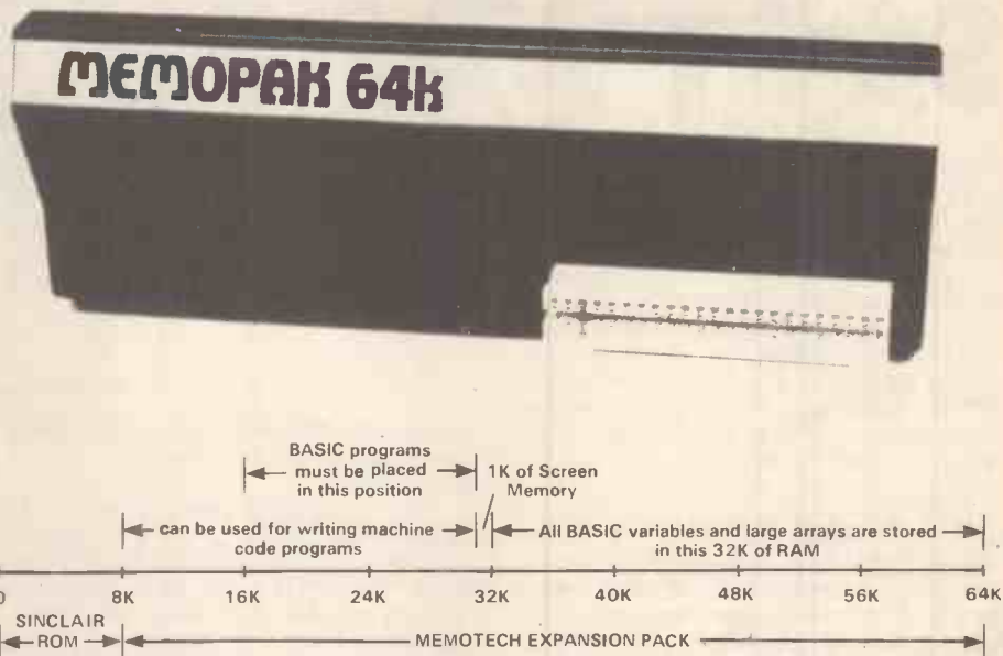
Figure 1. The layout of the 64K of memory available to the ZX-81 when used with the Memotech 64K RAM pack. Note that only about 15K is actually usable for BASIC program text. Note also, however, that 32K more is reserved for storing all the variables used in your programs and for large arrays of information. That 15K is thus actually far more powerful than it might seem!
