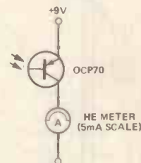
Figure 11.10. Testing a phototransistor with the HE meter.
