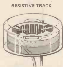
Figure 11.7b. The physical arrangement of a typical photoconductive cell.
