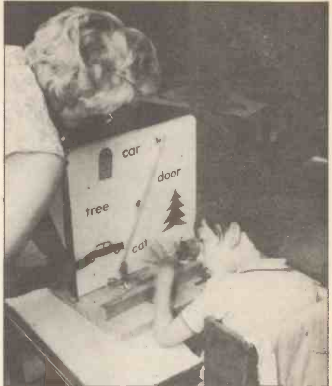
Early 'windmill' teaching aid in use. The spastic child can operate switches to make the pointer come to rest at the word which corresponds to the picture being indicated. The machine is made from Meccano components and is battery-operated
