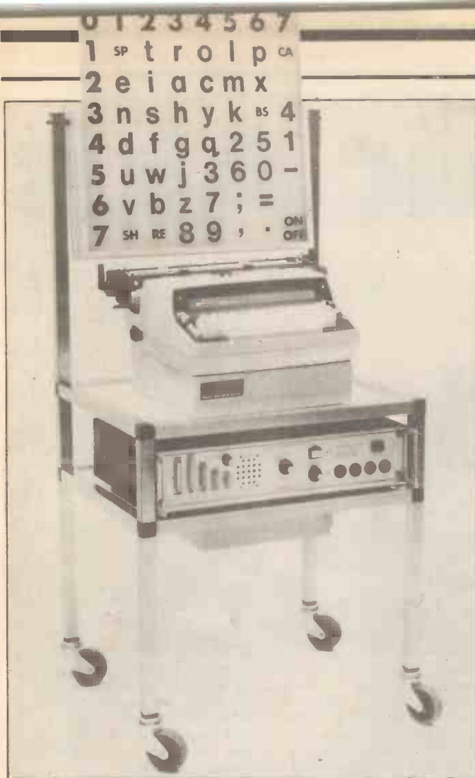
Electraid Typewriter Control 5600, with visual indicator, Brother large-print typewriter and trolley. It incorporates the facility for one, two or up to eight switch inputs
