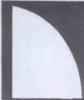
Power wave of full length non-loaded antenna
