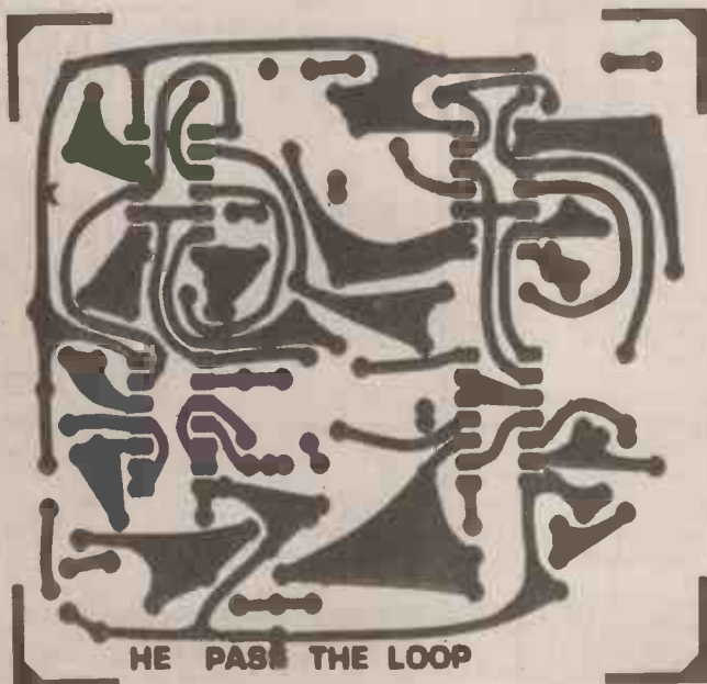
Fig 2. The foil pattern for HE Pass the Loop
