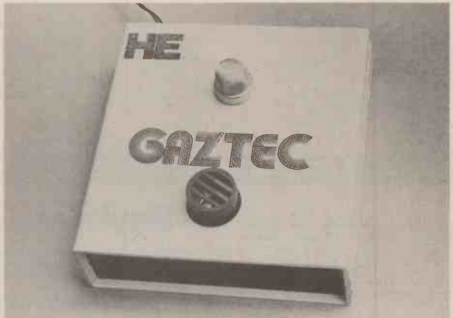
This good looking piece of electronic wizardry could end up saving your life one day. The metallic "nose" at the top is the gas sensor and the round black object underneath it is the solid state alarm.
