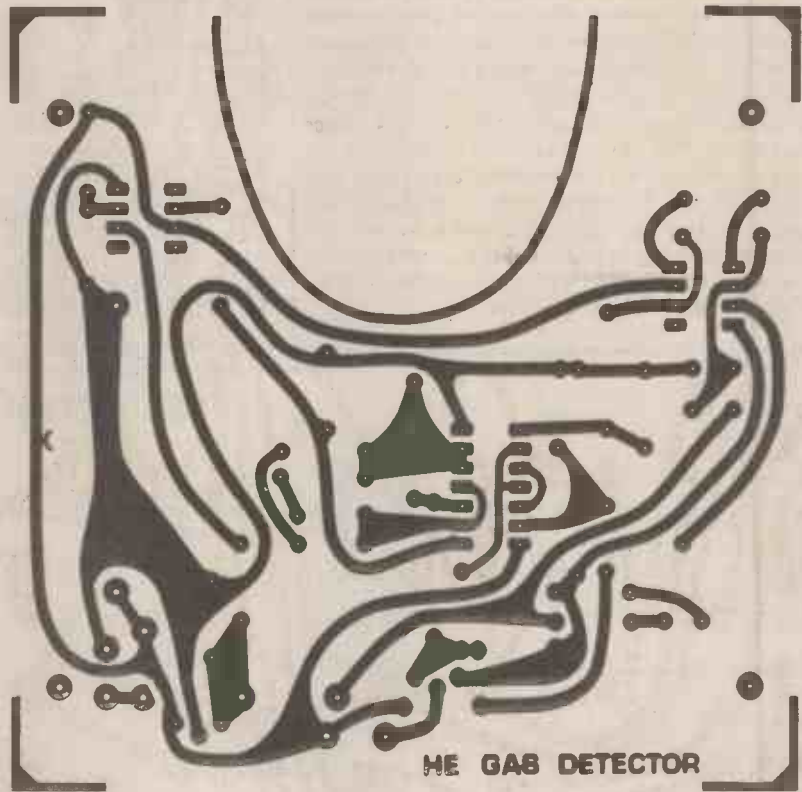
Figure 1. The foil pattern for the HE Gaytec
