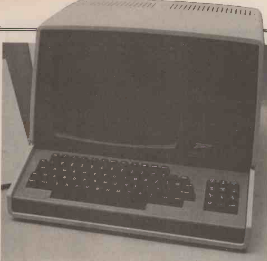
Above: the end result. This particular computer is a Zonith Z89, which uses two MPUs — one is there just to make the keyboard more efficient and easier to use. Printer interface is built-in too.
