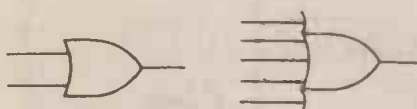
Above: truth table and circuit symbol for an OR gate. As with the AND gate, ICs are readily available containing four dual-input circuits in one package.
