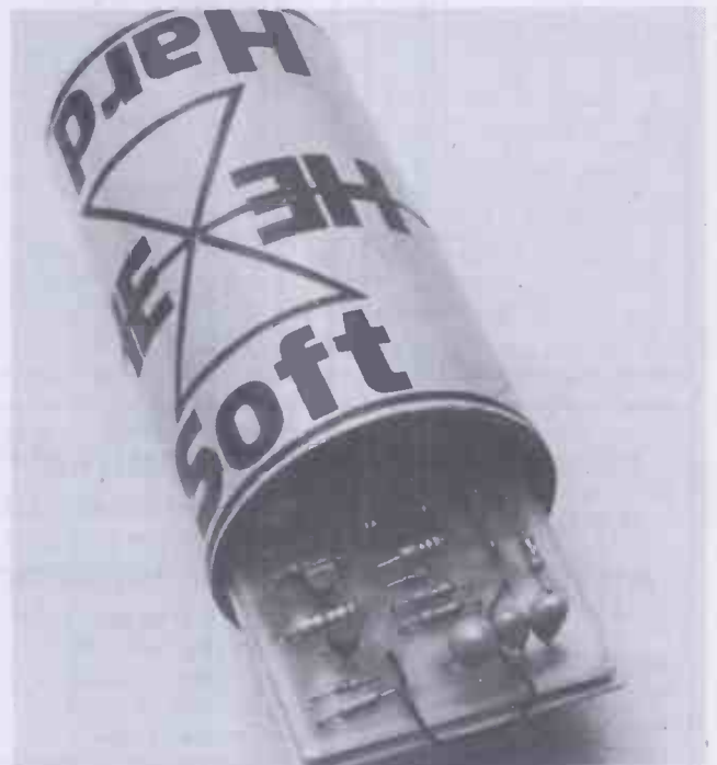
The HE Egg Timer in its 'swish' case made from a cardboard mailing tube. All the components fit neatly onto the main board.
