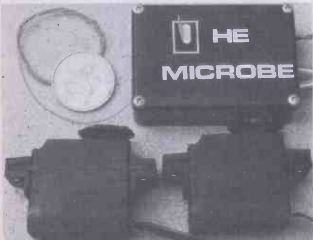
The Microbe receiver in its box. As you can see we cut a slot in the box to allow for easy changing of crystals.
